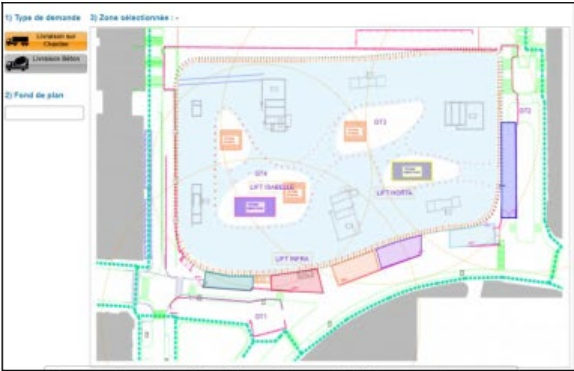
Example of online booking of lifting equipment
